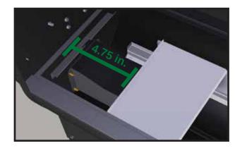
Improper shield placement will result in issues coming to temperature. When using the heat shield adjustment rod, a centered heat shield should be positioned approximately at the "0" mark on the rod, setting the heat shield roughly **4.75 in. (120.65 mm)** from the left inside grill wall. The depth to which the rod is threaded into the receiving nut varies, so some experimenting might be needed to find the perfectly adjusted center point on your rod.
