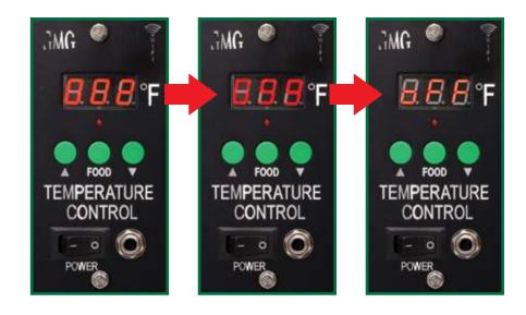
After you toggle the grill, the system will install the update and verify if it is installed correctly. You will see the grill count from "000" to "100" during this time. When the update is complete the grill will display "off". It will then disconnect from your local network and broadcast via the GMG network again.
