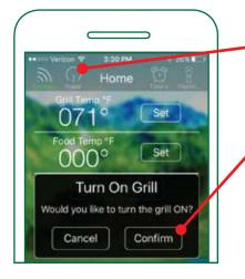
**ON:** First make sure you are connected to the grill. Once you verify you have power tap the "Power" button. A pop up screen will display. Press the "Confirm" button to turn the grill on.
