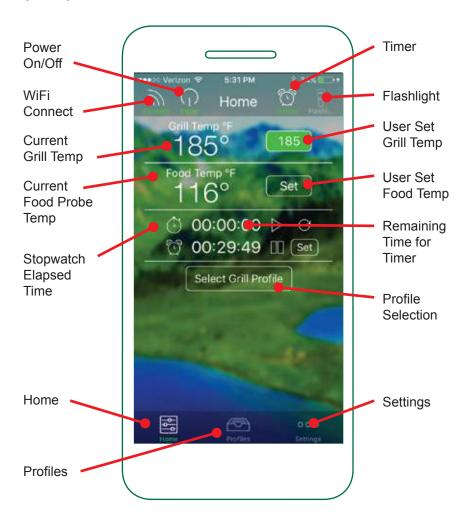
The control screen allows you to turn your grill on/off, set the grill temperature, set food probe temperature, set a timer and/or stopwatch.
